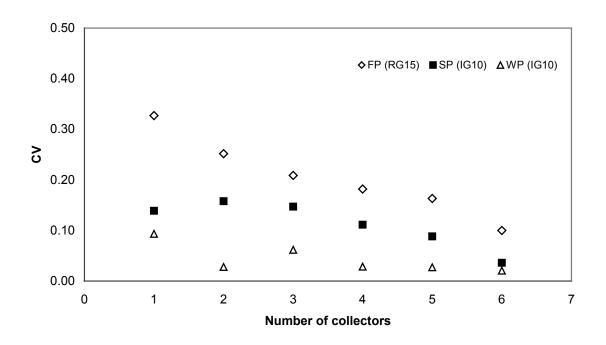
Figure 5. Effect of number of RG15 and IG10 collectors on coefficient of variability (cv) of irrigation depth under the FP, SP, and WP type irrigation packages.
