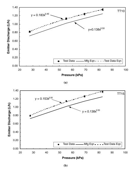
Figure 4. Emitter discharge/pressure relationships for the TT-10 product (a) and TT-15 product (b). The original discharge/pressure test data are displayed with error bars (±1 std dev) and the power function of those data. The discharge function from the manufacturers data is also displayed with that relationship.
