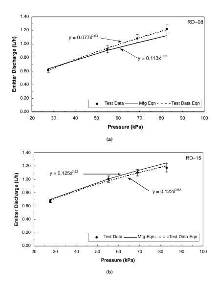
Figure 3. Emitter discharge/pressure relationships for the RD-08 product (a) and RD-15 product (b). The original discharge/pressure test data are displayed with error bars (±1 std dev) and the power function of those data. The discharge function from the manufacturers data is also displayed with that relationship.
