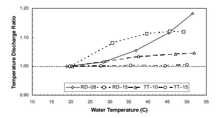
Figure 5. Temperature discharge ratio (TDR) values as affected by water temperature for the RD-08, RD-15, TT-10, and TT-15 products when operated at a pressure of 55 kPa.
