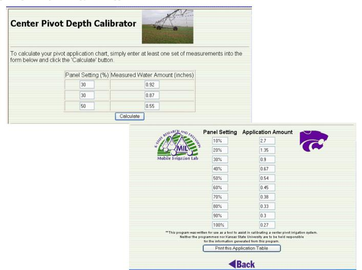
Figure 6. Screen shot of the online center pivot system application depth calibration program.
